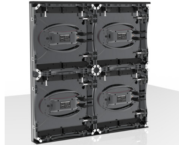
seamless fix installation cube 4x 90° r=1.2m | 5x 90° r= 1.5m
